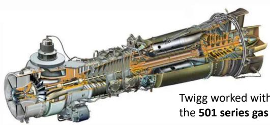
Twigg worked with Rolls Royce in developing various versions of the **501 series gas turbine engine** used for power generation.
